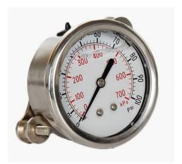
Application: Liquid filled pressure gauge mainly used in petroleum chemical industry liquid help to absorb vibration and pressure spikes, increasing the service life of the gauge.
