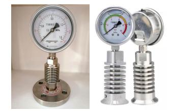
Diaphragm Seal Pressure Gauge is designed for pressure measurement that media does not directly contact instrument's measuring system and the pressure is transmitted through oil filled diaphragm seal unit. The sealed diaphragm would not raise a dead corner or area where residue may be left, which is universally used for sanitary applications. Plus the media is not contacted directly with the gauge sensor, so this type as well is suitable for high temperature and easy to block condition.
