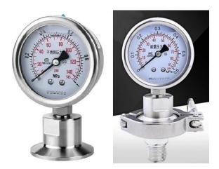
Diaphragm Seal Pressure Gauge is designed for pressure measurement that media does not directly contact instrument's measuring system and the pressure is transmitted through oil filled diaphragm seal unit. The sealed diaphragm would not raise a dead corner or area where residue may be left, which is universally used for sanitary applications. Plus the media is not contacted directly with the gauge sensor, so this type as well is suitable for high temperature and easy to block condition.
