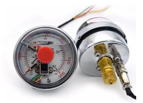
Model MYDJ series pressure gauge is a superior design type with electric contact controller output for pressure controlling and alarming in automatic process. When measured pressure reaches rated value, it outputs signals to operate auto-controlling and alarming device. It is suitable for measuring pressure of gas or liquid and characterized with novel design and reliable structure, good movement stability, durable installation and less maintenance.
