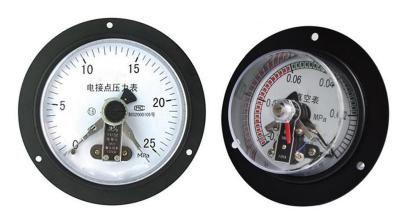
Model MYDJ series pressure gauge is a superior design type with electric contact controller output for pressure controlling and alarming in automatic process. When measured pressure reaches rated value, it outputs signals to operate auto-controlling and alarming device. It is suitable for measuring pressure of gas or liquid and characterized with novel design and reliable structure, good movement stability, durable installation and less maintenance.
