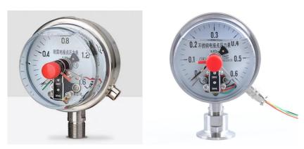
Model MYDJ series pressure gauge is a superior design type with electric contact controller output for pressure controlling and alarming in automatic process. When measured pressure reaches rated value, it outputs signals to operate auto-controlling and alarming device. It is suitable for measuring pressure of gas or liquid and characterized with novel design and reliable structure, good movement stability, durable installation and less maintenance.
