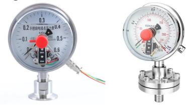
Model MYDJ series pressure gauge is a superior design type with electric contact controller output for pressure controlling and alarming in automatic process. When measured pressure reaches rated value, it outputs signals to operate auto-controlling and alarming device. It is suitable for measuring pressure of gas or liquid and characterized with novel design and reliable structure, good movement stability, durable installation and less maintenance.
