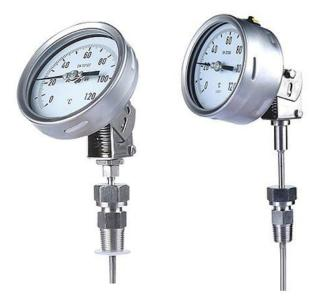
**WSS** series bimetal thermometer is a temperature-measuring instrument in which the differential thermal expansion of thin dissimilar metals, bonded together into a narrow strip and coiled into the shape of a helix or spiral, is used to actuate a pointer and to show the temperature value. It is also known as differential thermometer. Facilitated with all stainless steel material, it is suitable for corrosive media and environments in chemical process, petroleum and other industry field.
