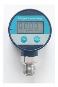
Digital Pressure Gauge is an intelligent pressure gauge with high precision, tracking speed, simple operation and reliable self-protection function. The product applies whole electronic structure and silicon piezoresistive sensor chip, with powerful anti-jamming capability, fast sampling speed, digital filtering techniques to ensure its high accuracy, low drift, reliable performance, anti-corrosion, anti-vibration, long life, and self-protection function.
