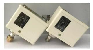
MC2020 universal pressure switch is a kind of pressure switch with ingenious structure and flexible use. It is equipped with bellows and mechanical mechanism. When pressure rises or falls, the corresponding mediation springs and ripples produce stretch or contraction displacement, and then push the switch through the lever action, cut off or switch on the control loop.
