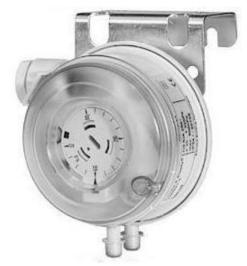
MC204A Air Differential Pressure Switch can be used to measure the pressure difference, vacuum or air flow of non corrosive gas and output NC+NO switch control. It is featured a wholly mechanical structure which is reliable and flexible in use.
