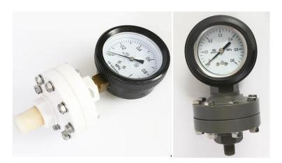
Diaphragm Seal Pressure Gauge is designed for pressure measurement that media does not directly contact instrument's measuring system and the pressure is transmitted through oil filled diaphragm seal unit. The sealed diaphragm would not raise a dead corner or area where residue may be left, which is universally used for sanitary applications. Plus the media is not contacted directly with the gauge sensor, so this type as well is suitable for high temperature and easy to block condition.
