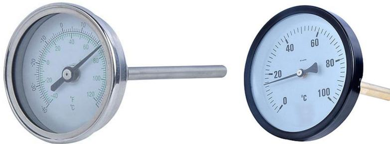
**WSS** series bimetal thermometer is a temperature-measuring instrument in which the differential thermal expansion of thin dissimilar metals, bonded together into a narrow strip and coiled into the shape of a helix or spiral, is used to actuate a pointer and to show the temperature value. It is also known as differential thermometer. Facilitated with all stainless steel material, it is suitable for corrosive media and environments in chemical process, petroleum and other industry field.
