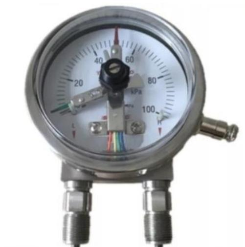
Differential pressure gauge with manifold valves:
